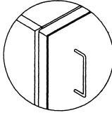
Drawers Constructed of 1/2" Particle Board Substrate & 1/4" Tempered Hardboard Bottoms and feature 8mm Hardwood Dowel Construction. All Exposed Surfaces are finished in White Melamine Laminate.
