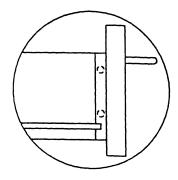
Toebases are furnished Unfinished and offered: Attached - Constructed Separately from 3/4" Particle Board Substrate & attached to the case at the factory (or)
